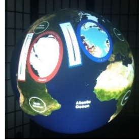
Figure 4: CoralTouch , a multi-touch spherical display prototype.
